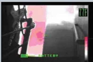
FAR LEFT: During the heat-release experiment, researchers determined that when a window was left open in the fire room, flame length out the window was smaller during natural ventilation (shown) than when using PPV fans to ventilate the room.
