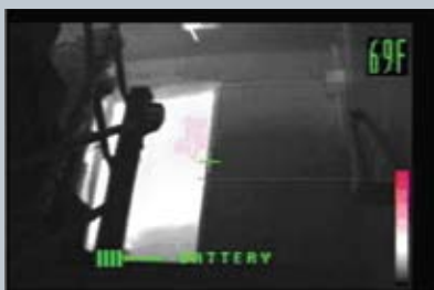
LEFT: In the thermal image above, hot gases are entering the stairwell through the open doorway. After the PPV fan was started, hot gases stop entering the stairwell, as shown in the image below.
